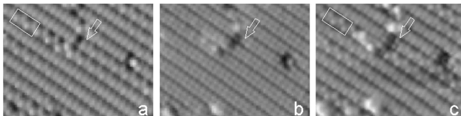
FIG. 4. Sensitivity of STM images of Si(100) to bias voltage. A filled-state image (a) [ -2.0 \text{ V} ] and two empty-state images taken with sample biases of (b) +2.0 \text{ V} and (c) +0.8 \text{ V} . White frames show the same area. Arrows point to an identical dimer in the vicinity of a missing-dimer defect; the dimer appears symmetric and can only be distinguished from others in (c). Image size: 85 \times 65 \text{ \AA}^2 .
